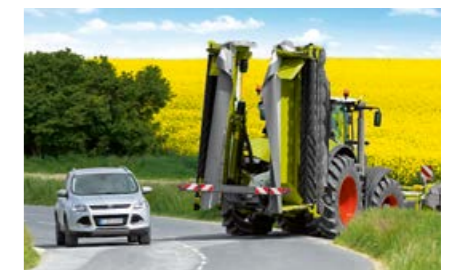
Less than 4.0 m: compact transport position with generous ground clearance in both BUSINESS models
