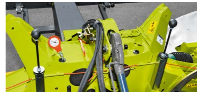
Pressure-gauge dial to conveniently set the ground pressure for both mowing units
