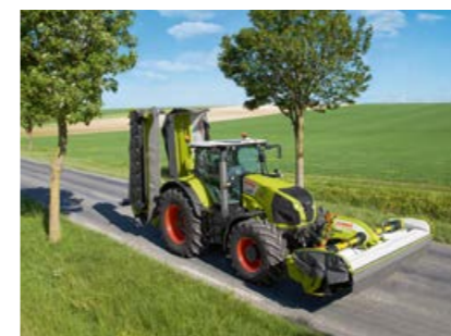
Compact transport position for safe road travel
